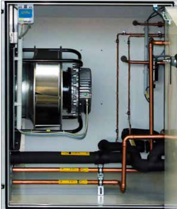
EC fan module (ebm-papst), standard design with spider (vibration-decoupled mounting on the pressure bulkhead).
